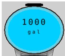
The tank capacity indicator will display the remaining tank volume.
