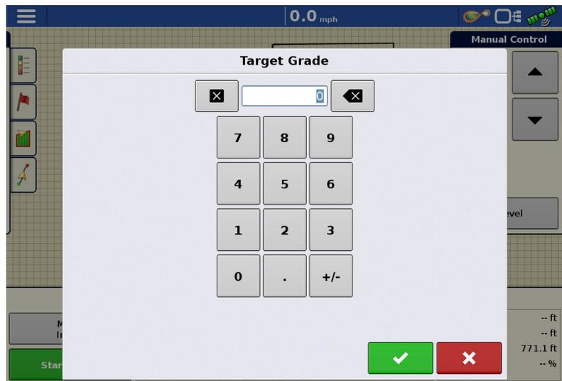
**Target**—Use this button to select the grade you desire. You can change this setting on the fly, and Intellislope will follow the new grade starting at the point when the Target grade changed.
