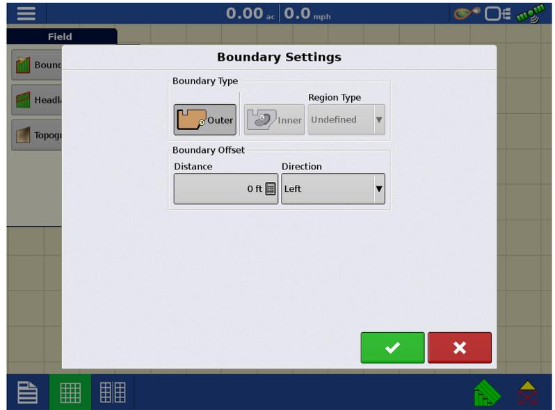
1. Choose whether to create either an Outer boundary or Inner boundary by pressing one of the two Boundary Type buttons.
