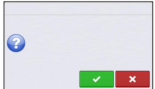
10. After pressing the green check mark the mobile device will begin accepting data from the display as it becomes available. The AgFiniti Status Indicator will show a device symbol in the top right corner of the screen. Note: If display is logged in to AgFiniti Cloud a cloud symbol will also appear in the AgFiniti Status Indicator.
