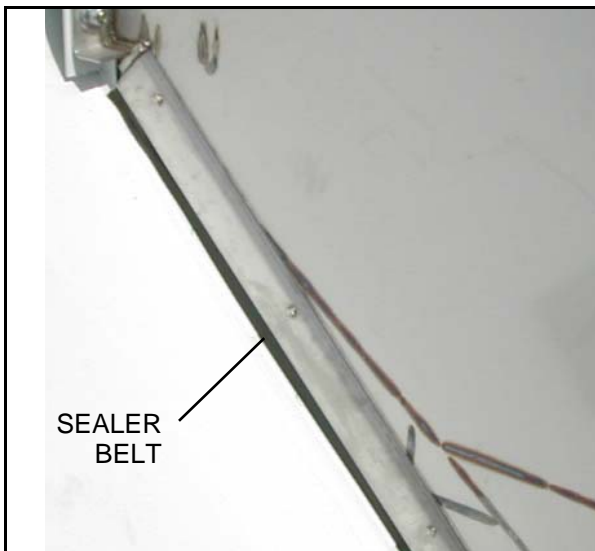
Figure 12 – Front Sealer Belts
