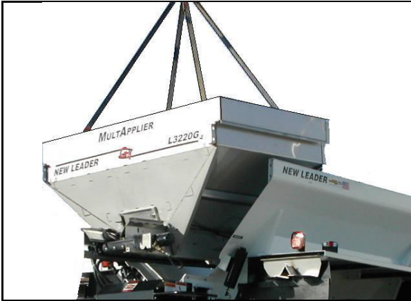
Figure 11 – Four-Point Lift
